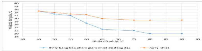
Figure 11. Correlation between oil treatment temperature and freezing temperature of oil achieved after thermal treatment
