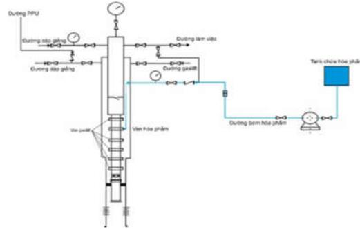
Figure 12. Chemical pump pipe installation principal diagram
