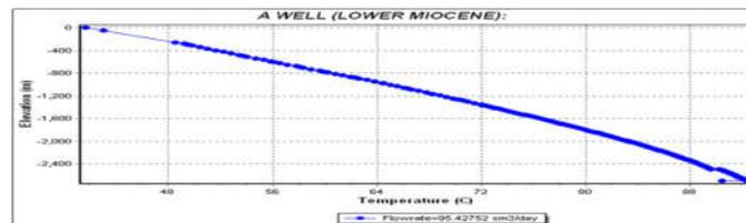
Figure 13. Gradient well temperature A with  $Q=95 \text{ m}^3/\text{day}$
