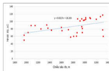
Figure 9. Temperature dependence on the depth of the Miocene object
