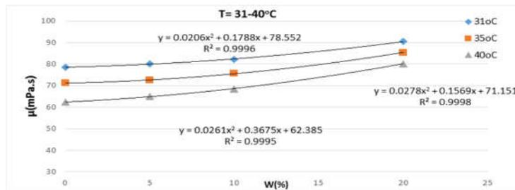
Figure 5 – Crude oil viscosity vs water saturation under temperatures of 31-40oC 31-40°C
