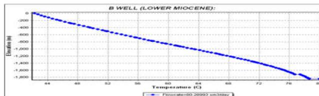
Figure 14. Gradient well temperature B with  $Q=80\text{m}^3/\text{day}$
