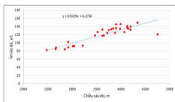
Figure 8. The dependence of temperature on the depth of the basement object
